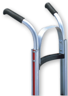
TYPE 16 HANDLE Standard double pistol grip handle. Curved out to meet the operator's hands for two-handed control. Model # 16
